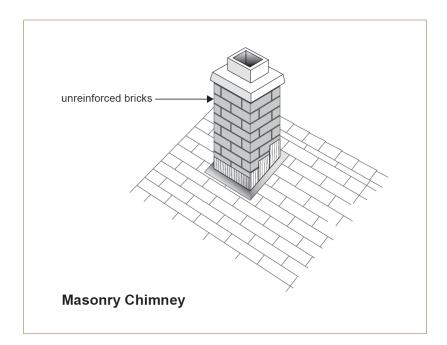
Unreinforced masonry chimney may collapse, striking occupants below or damaging roof and other structural elements supporting the building.
