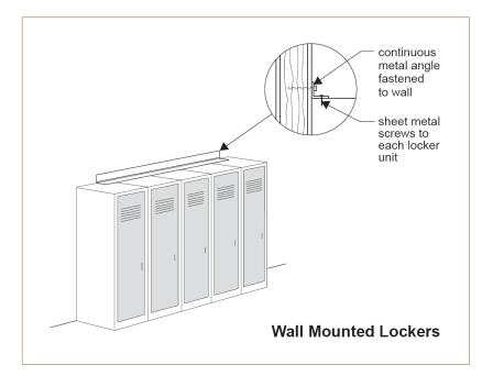
Unsecured wall mounted cabinets/lockers (shown)/coat closets may fall, striking nearby occupants or blocking hallways and exit ways.
