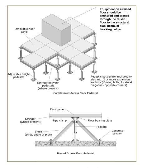
Equipment mounted on access floor (modified from: FEMA E-74).
