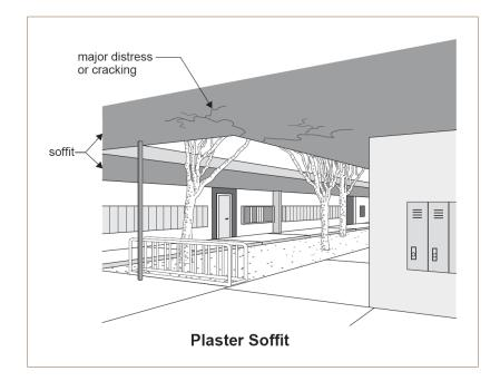
Plaster that is cracked, deteriorated, or was installed prior to 1978 may collapse; striking occupants below or blocking hallways and exits during an emergency.
