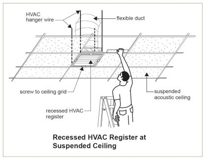
Unsecured ceiling mounted light fixtures and HVAC registers may fall, striking occupants below or blocking exit ways for evacuation during an emergency.
